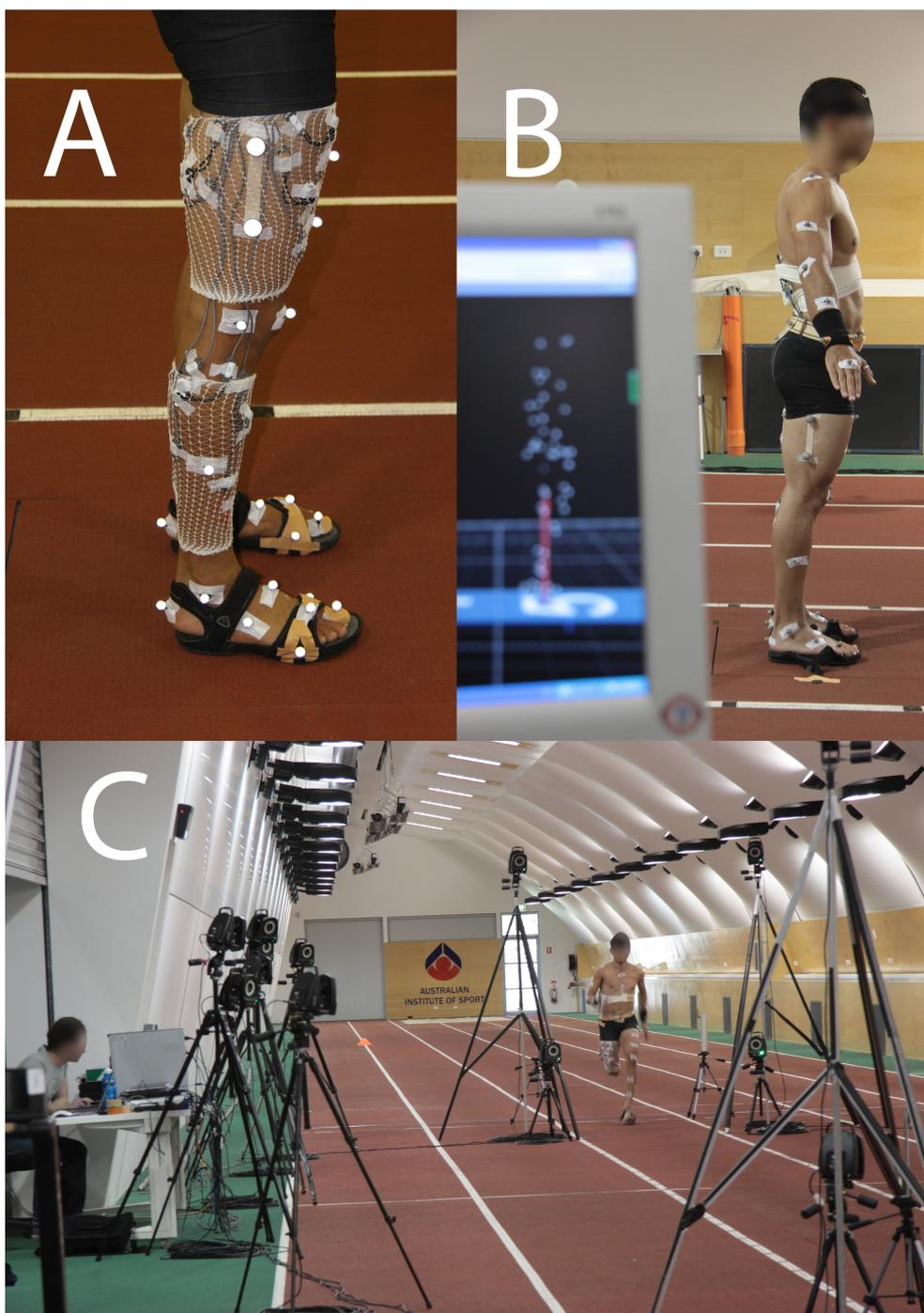
**Figure 3.3:** *Experimental data capture photos. (A) a prepared leg containing markers and EMG electrodes. (B) capture of a static trial. (C) capture of a running trial at 7.0 m/s.*
